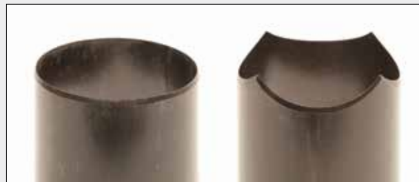
Outside sharpened: push up native soil
